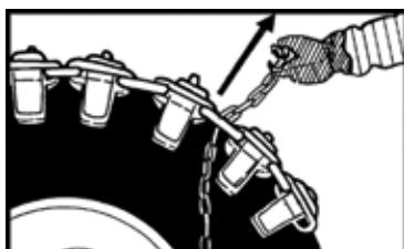
Insert the other end of the mounting chain through one of the longer track links on the top section. Pull the chain tight.
