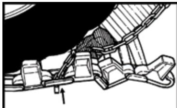
Insert the mounting chain through one of the longer track links on the ground section (see illustration).
