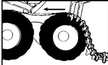
Roll out the track and join the 2 sections with the long track locks included in the joining set. Drive over the track and bring the other end over the top of the tires so that both ends are at one end of the bogie.
