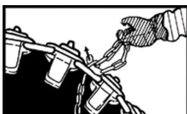
Lock the chain by inserting the free end through a link as shown. After both chains are installed, check that they have the same length on either side. Drive forward until the chains are between the bogie wheels. Connect the track ends together with the track locks included in the joining set.
