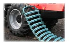
Position the machine so that the wheel is lined up with the track and wrap the chain around the centre of the tire. Place the loose end of the chain on ground in front of the tire.
