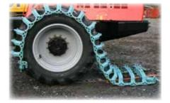
Pull the track around the top of the wheel by driving over the chain.
